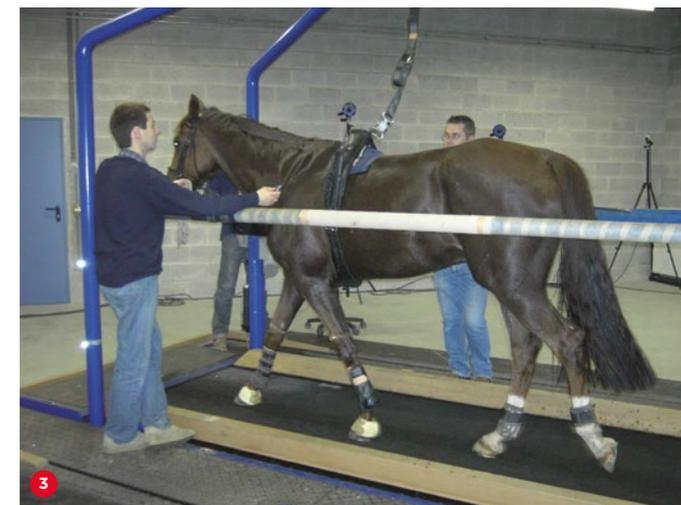
**Cameras register the horse dynamic simultaneously. Results are analyzed by computers and adapted programs (fig. 4).**
